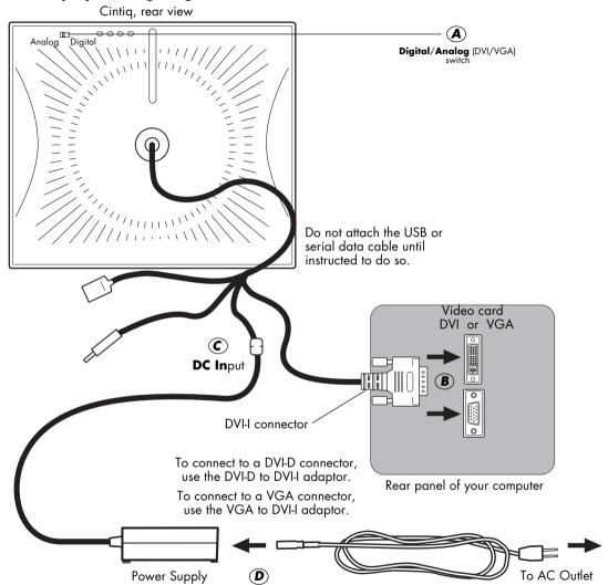
CAUTION Make sure that you correctly set the Cintiq Digital/Analog (DVI/VGA) switch for the video card you are using.
