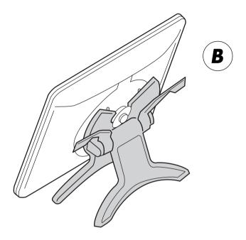
WARNING When operating the incline adjustment levers, Cintig must be mounted on the stand with the  $\Lambda$ stand feet resting on a stable, flat surface. The stand is spring-loaded and can snap back quickly, causing injury or damage if not operated properly.
