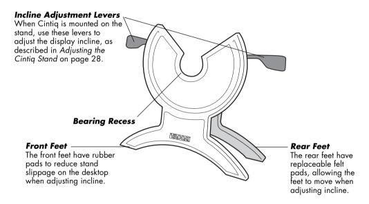
The Cintig stand supports the Interactive Pen Display unit. The stand can be used to adjust the incline angle of the display unit from a low position (13 degrees from horizontal) to a high position (70 degrees from horizontal). And, you can rotate Cintig from landscape to portrait orientation, or to any angle between +180 and -180 degrees. The stand also allows easy removal of Cintig for use in a semi-supported lap position.
