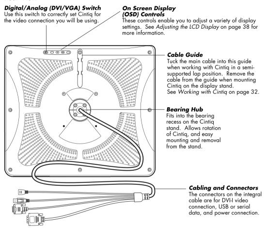
**Important:** Always store the Interactive Pen Display on the Cintiq display stand or in its original packing carton when not in use. Do not store the display unit on a flat surface that would excessively bend or crimp the cable.
